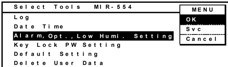
2. The Alarm, Option, Low Humidity Setting screen is displayed. On this screen, the temperature alarm (Temp Alarm), delay time of alarm (Alarm Delay), alarm resume time (Ring Back) and lamp (Lamp) can be set. The alarm buzzer is silenced by pressing the alarm buzzer stop key (BUZZER) during alarm condition. The buzzer will be activated again after certain suspension if the alarm condition continues. The suspension time (ring back) can be set.
