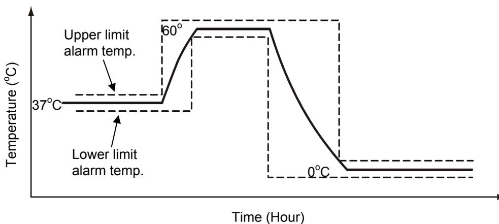
\* The buzzer is stopped by pressing the alarm buzzer stop key (BUZZER), but the remote alarm keeps alarm status. The buzzer resulting from upper limit alarm and lower limit alarm cannot be silenced by the alarm buzzer stop key (BUZZER).
