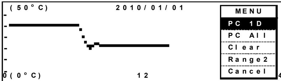
2. The Progress screen is displayed. Specify a transfer, capture of text and retention file name by operation of hyper terminal on PC. Apply "txt" or "csy" to retention file as an extension. Press the menu button (MENU) to show the menu window. Select "Start", and press the enter key (ENTER). The transmission is started. "Finished" display means the end of transmission.
