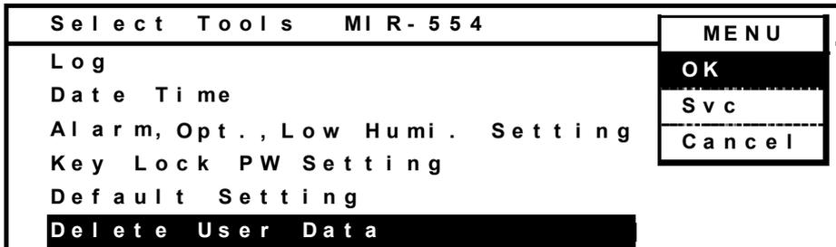
2. The Delete User Data screen is displayed. To select a program to deleted, select "Delete a User Program" and press the menu button (MENU) to show the menu window. Select "OK" and press the enter key (ENTER).
