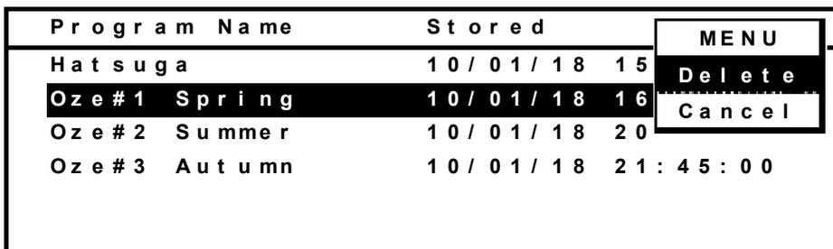
4. The Confirmation screen is displayed. Press the menu button (MENU) to show the menu window. Select "OK", and press the enter key (ENTER). The program (Oze#1 Spring) is now deleted.
