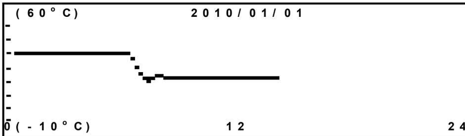
Similarly, select "Range1" and press the enter key (ENTER). Upper limit is changed from 60 °C to 50 °C and lower limit is changed from -10 °C to 0 °C.
