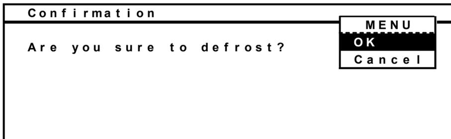
3. Press the menu button (MENU) to show the menu window. Select "OK", and press the enter key (ENTER). The manual defrost is started. During defrosting, "Defrosting" is displayed at the upper left on the top screen.
